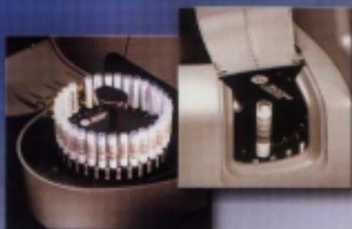
The FC 500 offers three modes of operation, from automated carousel to single-tube acquisition for maximum flexibility.
